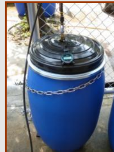
Internal pressure hydraulic test
